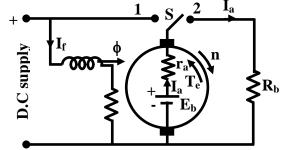
Figure 39.23: Machine operates as motor
