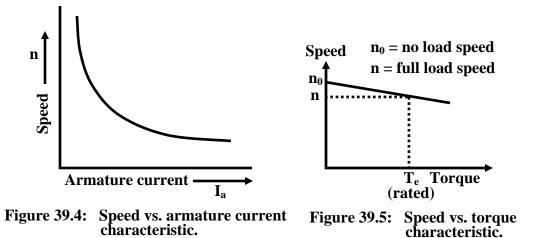
It is for this reason, a d.c shunt motor is said to be practically a constant speed motor (with no external armature resistance connected) since speed drops by a small amount from no load to full load condition.
