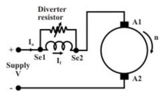
Figure 39.19: Field control with diverter.
