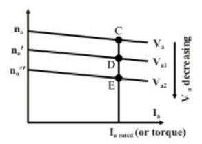
Figure 39.11: Family of n VS. I, characteristics.
