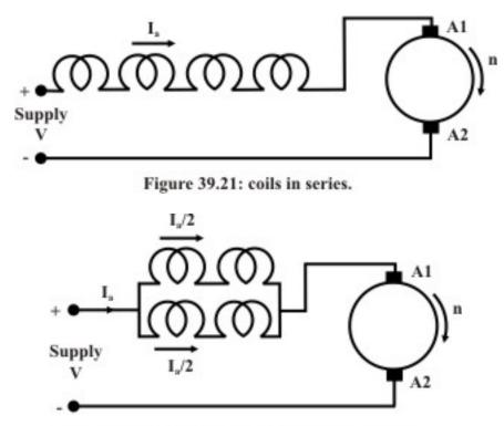
Figure 39.22: Series-parallel connection of coils.
