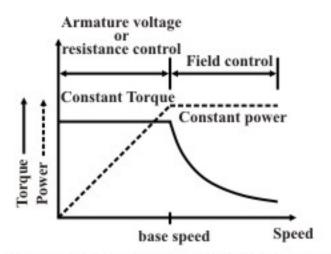
Figure 39.9: Constant torque & power operation.
