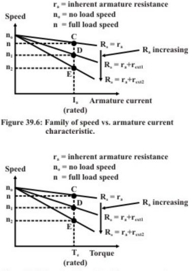
Figure 39.7: Family of speed vs. Torque current characteristic.
