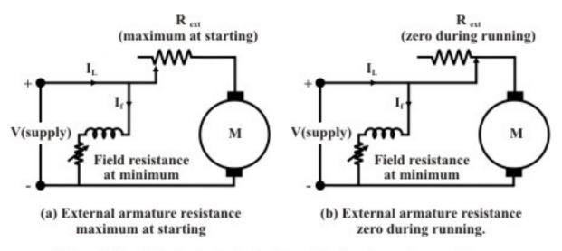
Figure 39.2: A simple starter in the form of external armature resistance.
