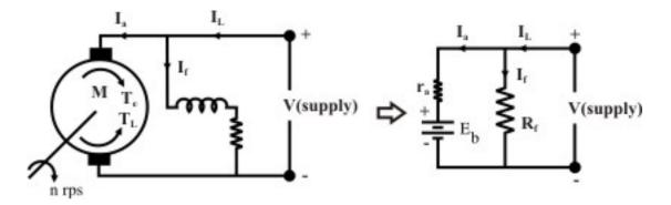
Figure 39.1: D.C shunt motor connection & its circuit representation.
