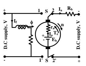
Figure 39.25: Machine operates as motor
