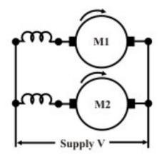
Figure 39.18: Motors connected in parallel.
