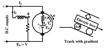
Figure 39.28: Machine enters regenerative braking mode.
