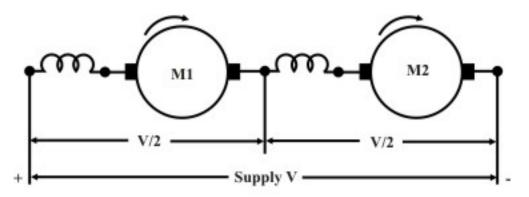
Figure 39.17: Motors connected in series.
