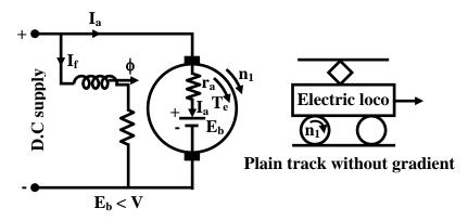
Figure 39.27: Machine operates as motor
