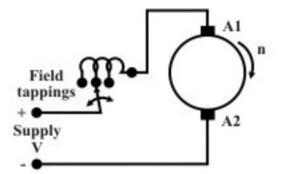
Figure 39.20: Field control with tappings.
